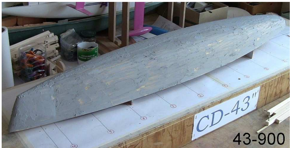
Epoxy filler all over the hull
