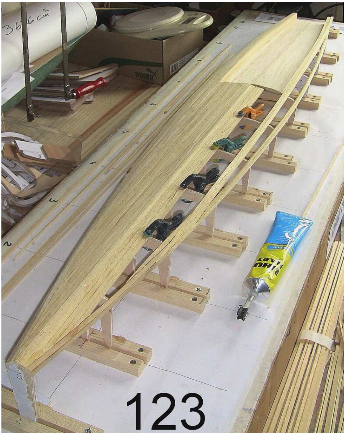
Deck strip planking seen from above
