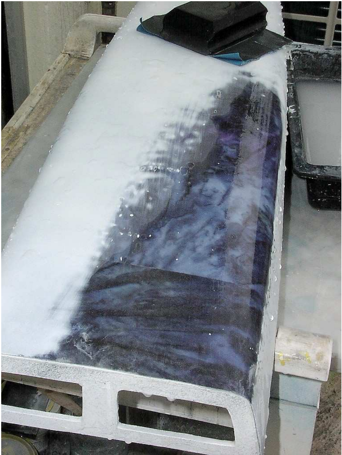
Progressive surface appearance during wet sanding
