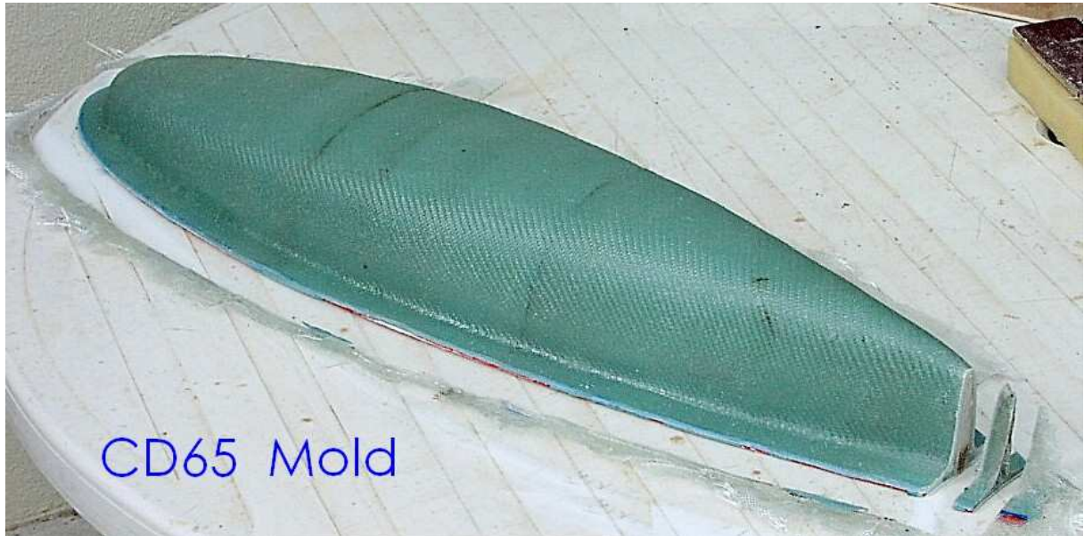
After 9 layers of fiberglass-epoxy of 200g/m 2
