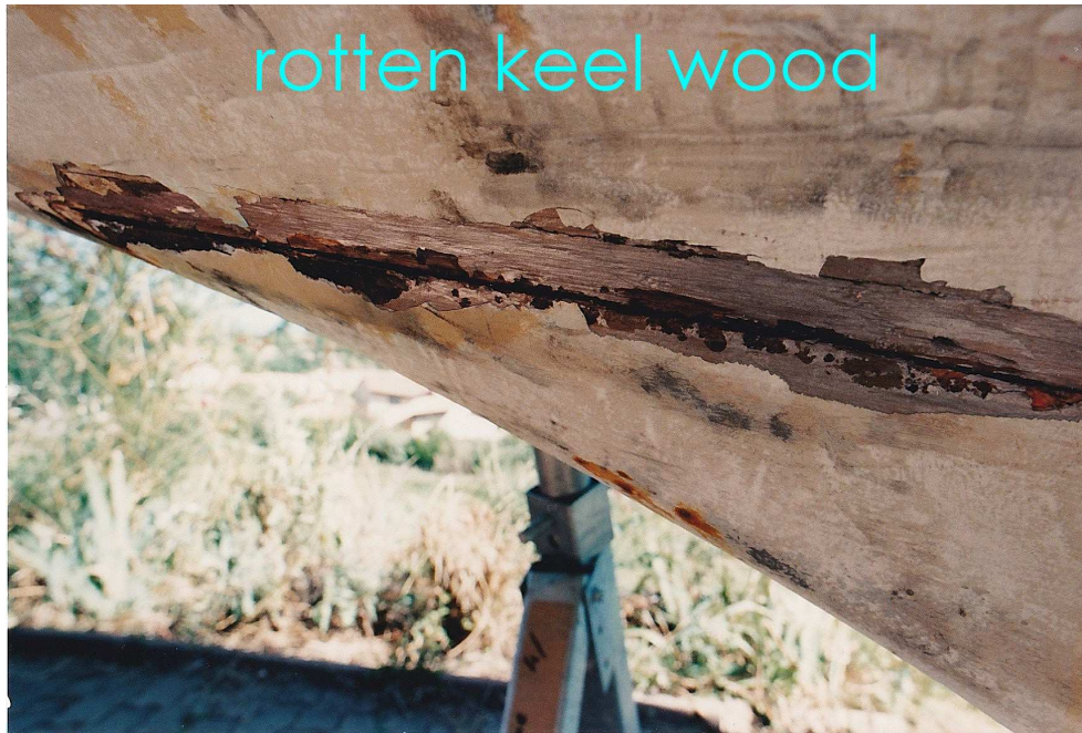
A lot of rotten wood needed replacement
