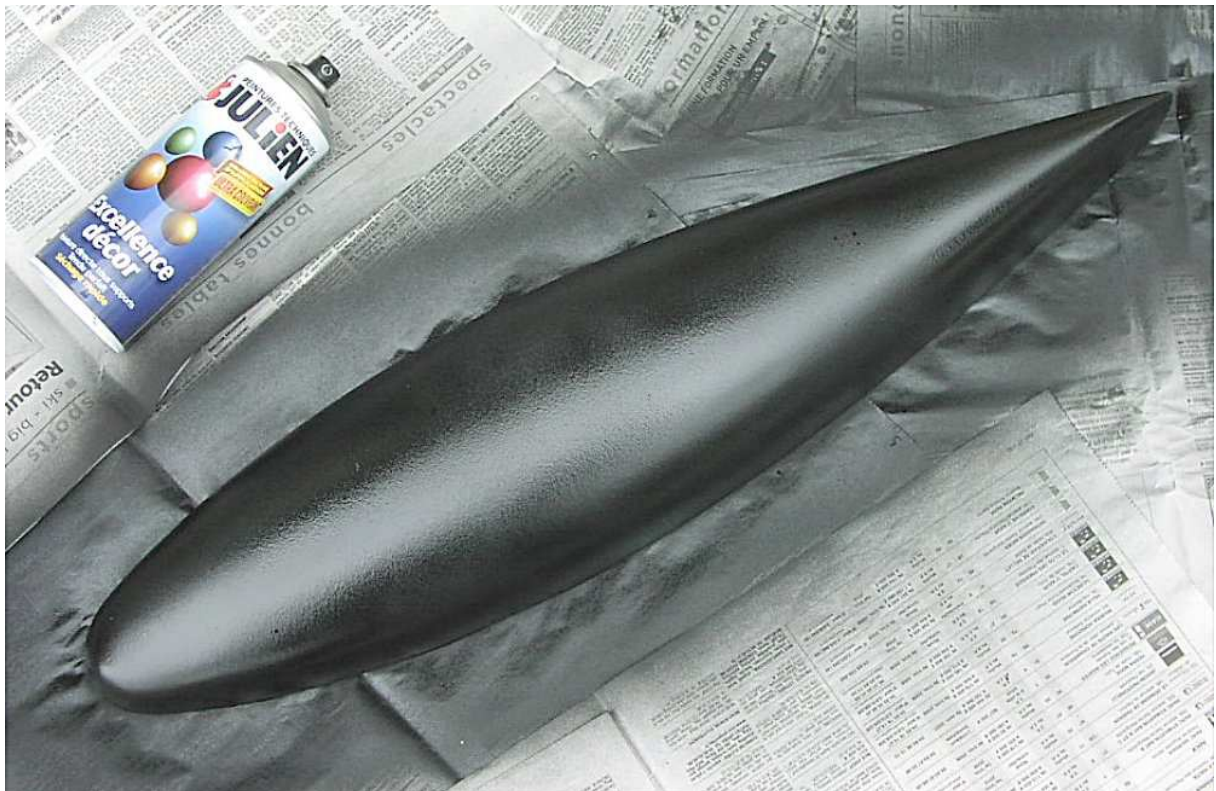
Several paint layers used, aiming to get best finish for the mold fabrication
