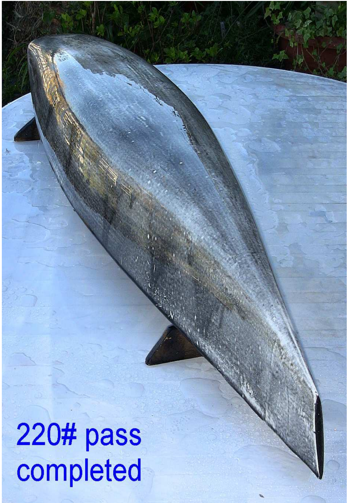
The Hull after wet sanding and ready for wax application
