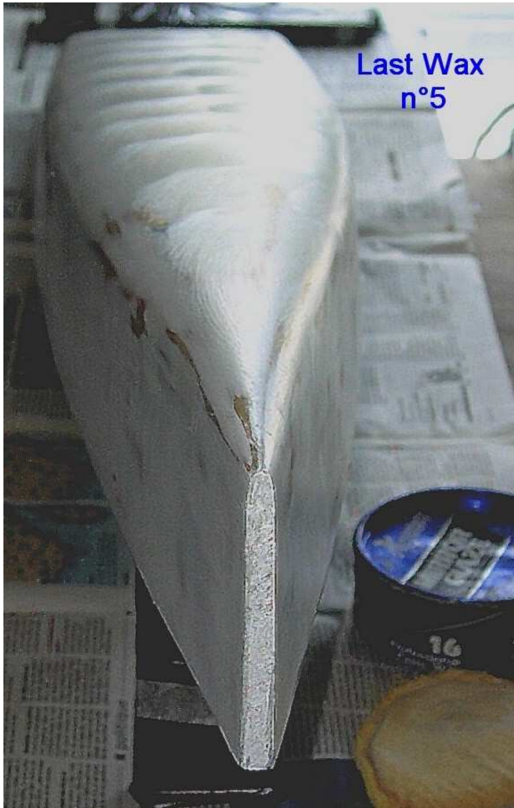
Before start hull lamination on male mold, several coats of wax are applied (here Mirror Glaze used)
