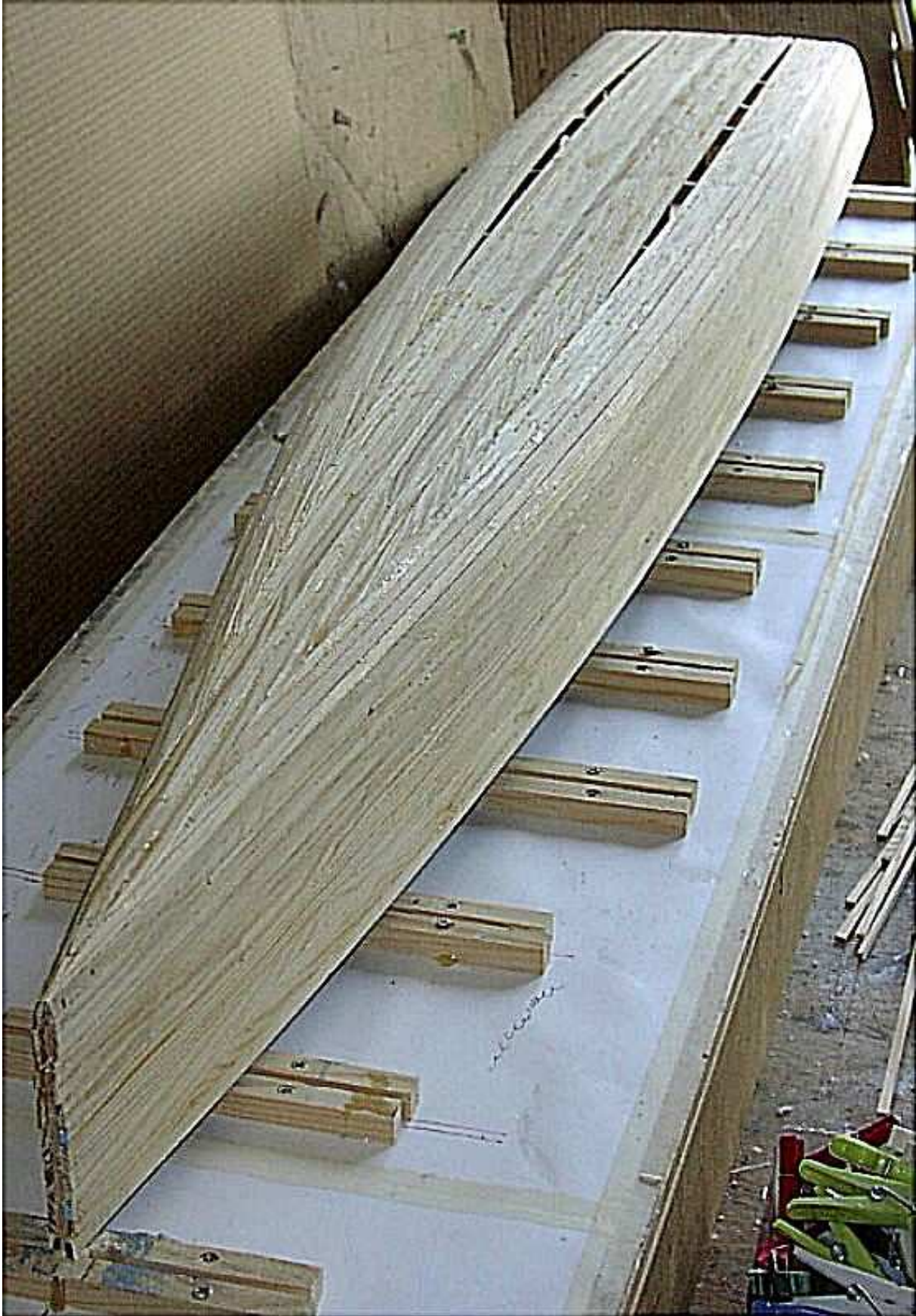
Strip Planking almost complete
