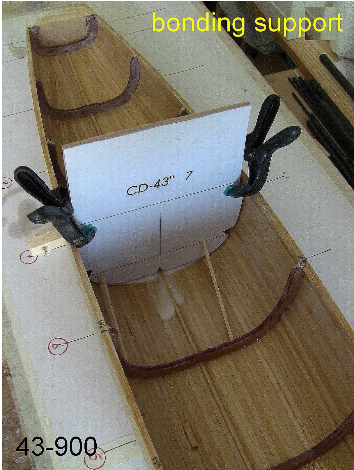
Supports used to allow external tissue laminations
